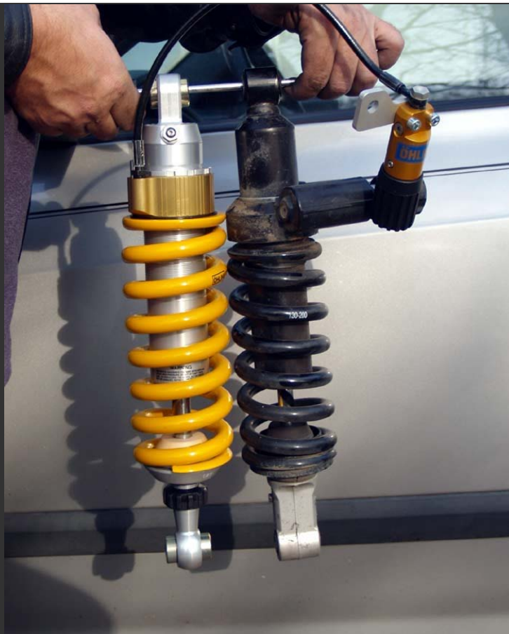
Stock shock compared to the Ohlins. The Ohlins was .5" shorter.
