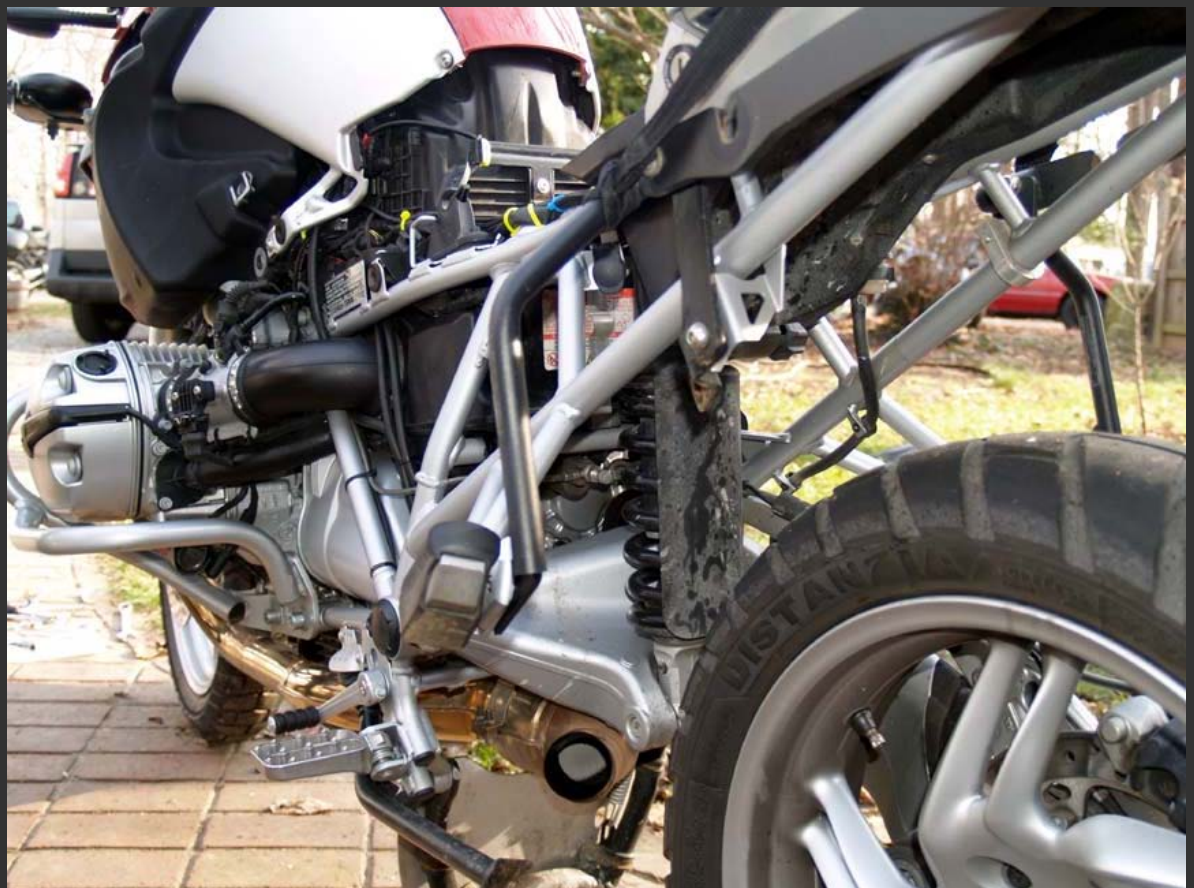
Remove the lower bolt T-50. In some cases this bolt uses red locktight so you must heat it to 200° to get it loose.
