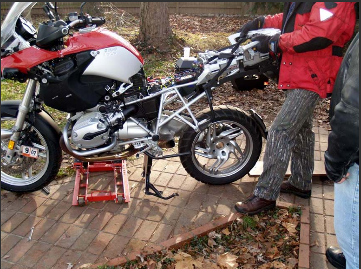
Have someone hold the bike steady, or strap it down. (Yes, this is after the shock was removed, but for illustration purposes.)
