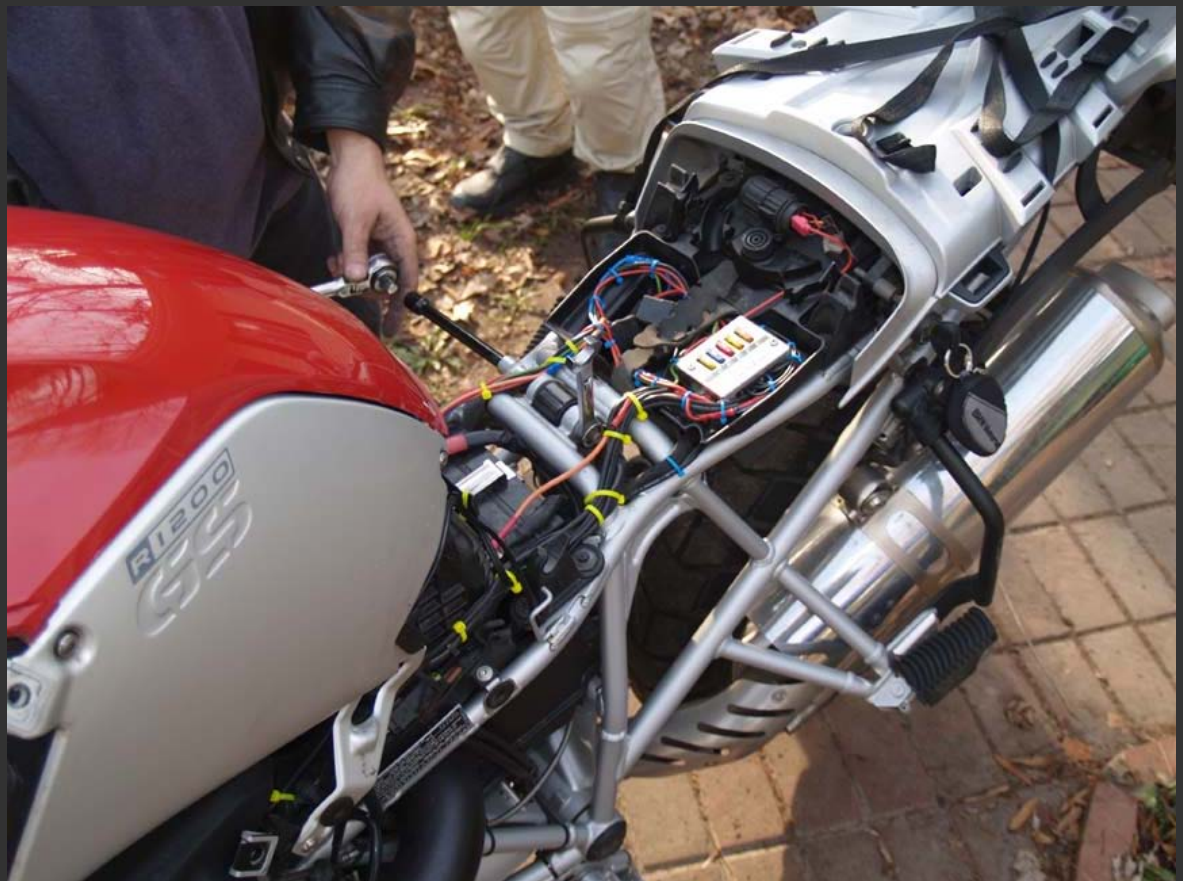
Loosen the upper bolt. T-45 and 16mm socket.
