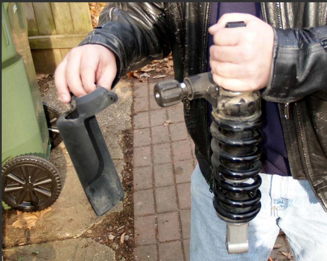
This is the upper nut, an oval locking nut.
