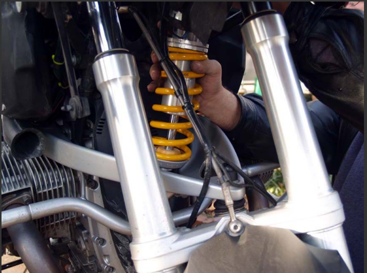
Carefully thread the shock past the wires and hoses. Note that the springs are larger around, and it makes it tight, but it fits. On the first bike we removed the belt cover to get clearance, but realized on mine that
