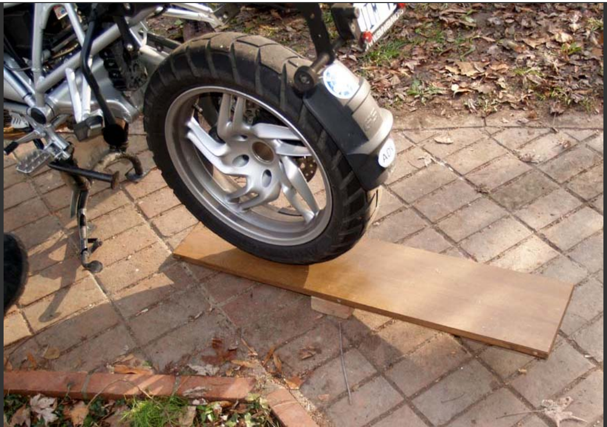
Prop the rear wheel so it doesn't drop when the shock bolts are removed.
